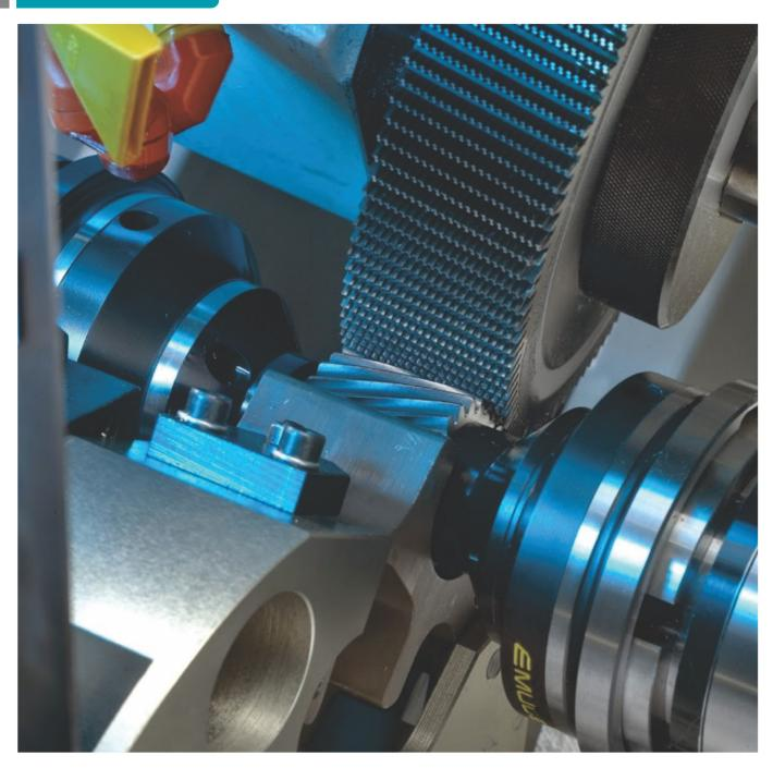
Spur & Helical gears can be supplied with various material configurations like - CK45/AISI1045, EN19, EN24, SAE 8620, EN 353, 16MnCr5, 20MnCr5 with gear shaving.
